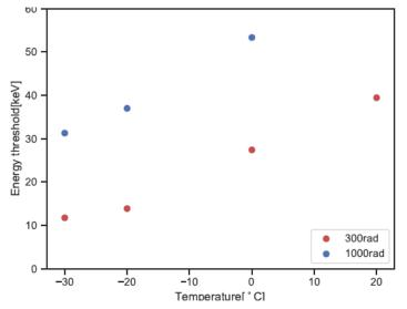
Comparable thresholds for both MPPCs with surface mounting.
