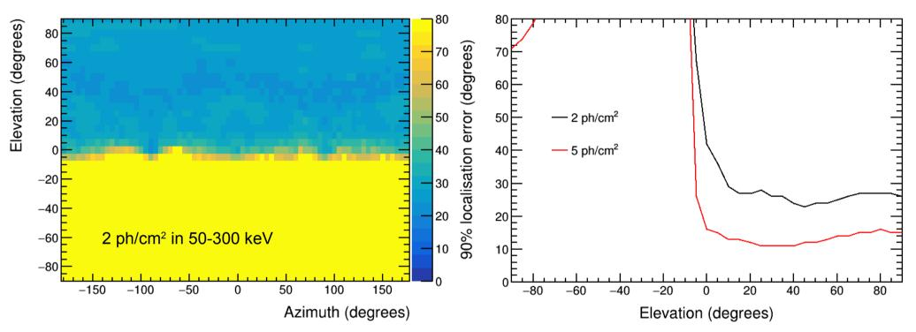
Above the instrument, the localisation error <  $30^{\circ}$  for 90% of the GRBs near the detection threshold (2 ph/cm<sup>2</sup>) and the localisation improves for brighter bursts.
