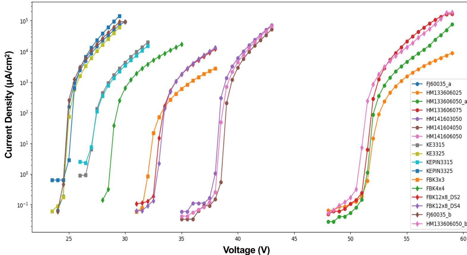
IV curves for the various SiPMs at one fluence ( $3.06E+10$  p/cm<sup>2</sup>) plotted as a function of voltage. Doesn't really show much since they all have different breakdown voltages. **Need to plot them versus overvoltage.**
