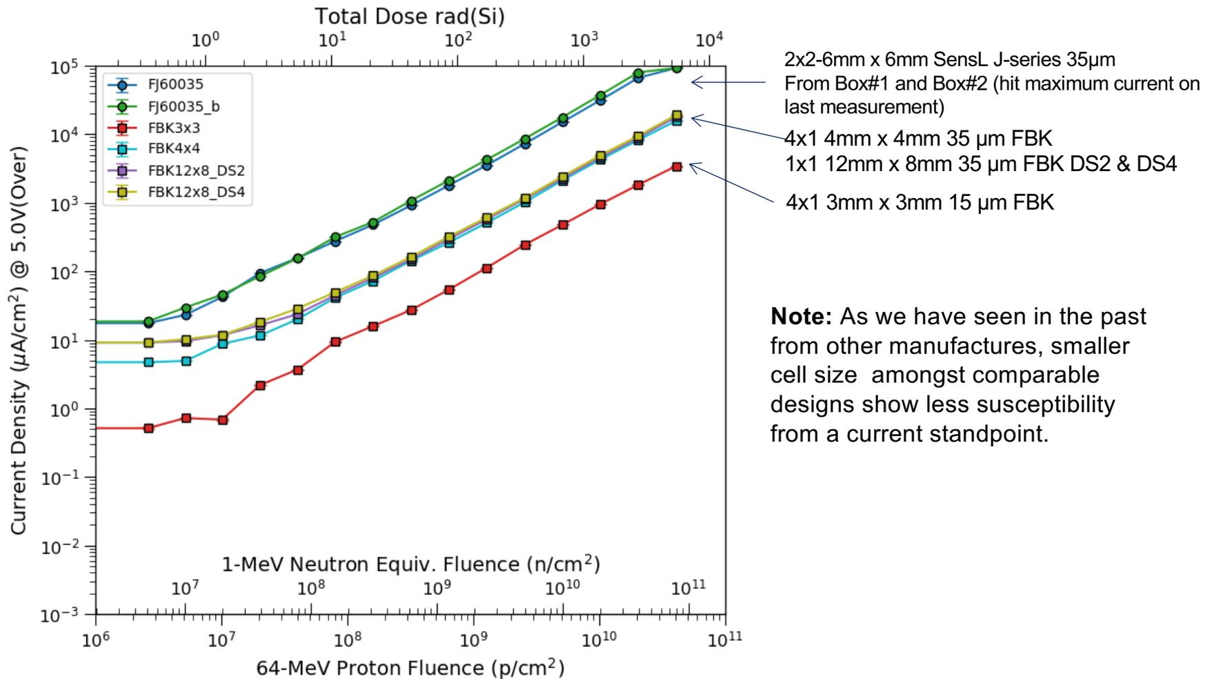
Plot of Current Density as a function of fluence(dose). Current is normalized by the active area (Note: we are considering active area to be the photosensitive area.)
