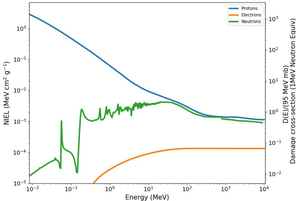
Non-ionizing energy loss as a function of energy for three particle types.
