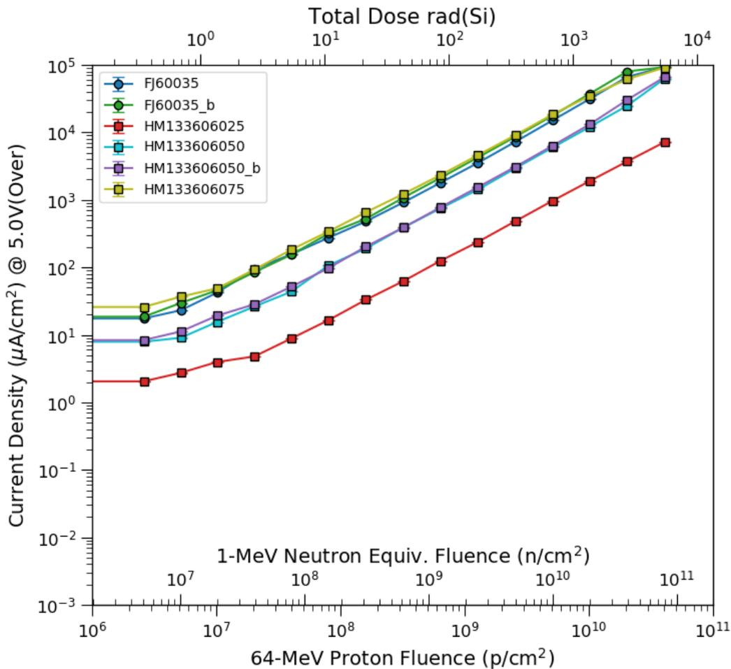
**Note:** As we have seen in the past from other manufactures, smaller cell size amongst comparable designs show less susceptibility from a current standpoint.
