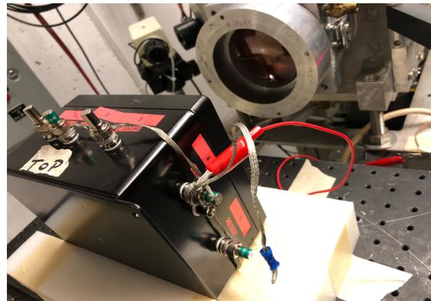
Test box in front of beam port. Laser alignment used to center target on beam. SiPMs ground during irradiation.
