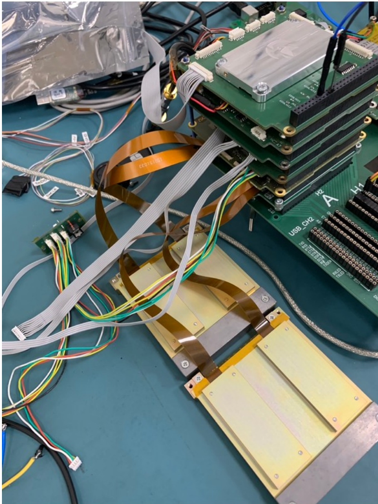
Tested that it operates on the satellite bus
