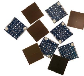
SensL MicroFJ-60035 SiPM chip (left) and the GRID SiPM array board (right)
